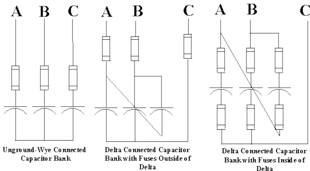
*Figure 1 -Connection and fusing arrangements for ungrounded-wye and delta connected capacitor banks*
